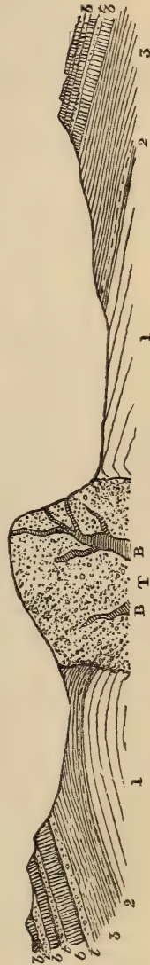
FIG. 289.—SECTION ACROSS THE BINN OF BUENTISLAND, FIFE. 1, Sandstones; 2, Limestone; 3, Shales, &c.; b b , Interstratified basalts; t t , Bedded tuffs, &c.; T , Tuff of the great neck of the Binn; B , Basalt veins.
